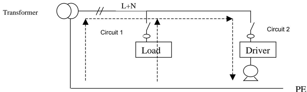
Figure 4: Influence of converter (driver) upon the load
