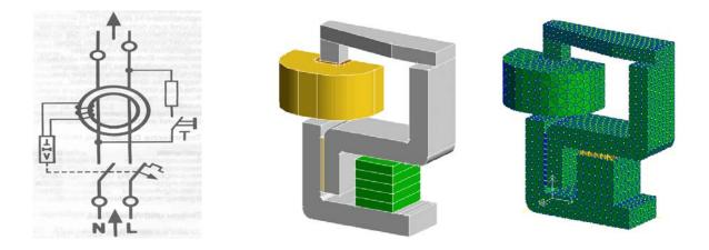
Figure 1: Wiring diagram of RCBO
