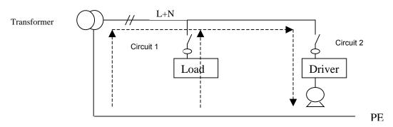
Figure 4: Influence of converter (driver) upon the load
