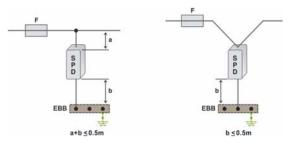
Picture 7: Proper installation and maximum conductor length
