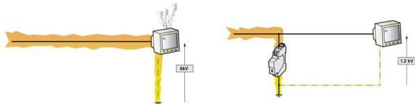
Picture 4: Voltage level without arrester
